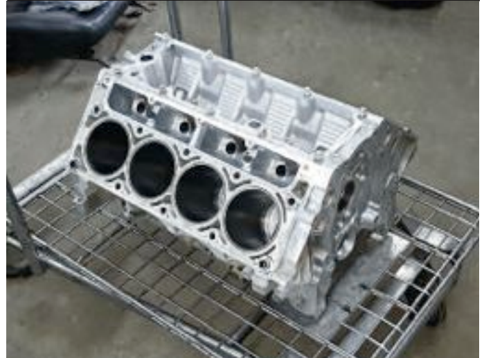
This aluminum LS block will soon get a full buildup. While iron blocks are everywhere, these are much more scarce.
