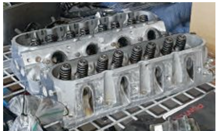
These cathedral-port LS1/LS2 heads are used and have been removed and inspected for obvious flaws. They will likely be rebuilt and pressed back into service in pretty short order. Ron and his staff have a very busy mail room and will ship worldwide.
