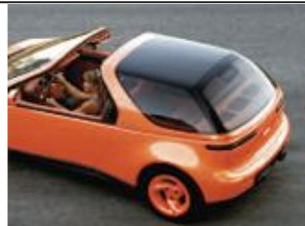
**Left: With its rear seat down and tailgate opened, the Salsa could easily serve as a light-duty pickup truck. Slide-out package tray saw production on the Aztek. Right: Removable wagon top added weather-tight storage space.**
