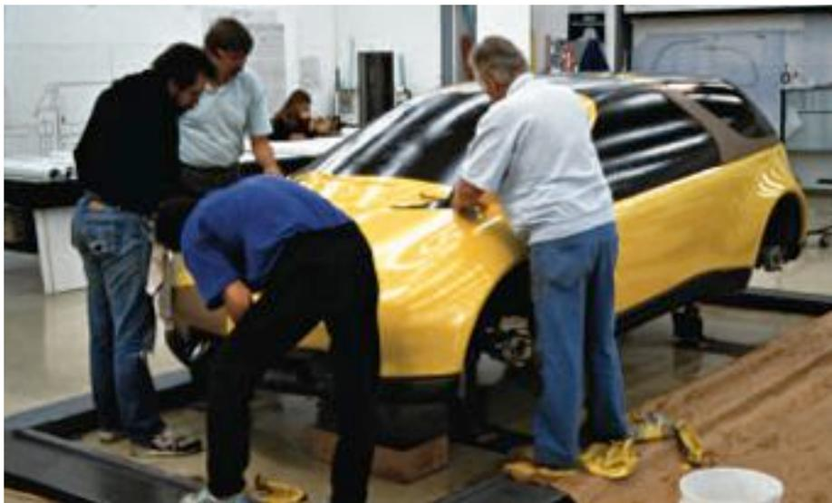
**The clay model is finished up with some bright yellow Di-Noc plastic sheeting to simulate a painted finish. This is an entirely different model than the turquoise showcar.**
