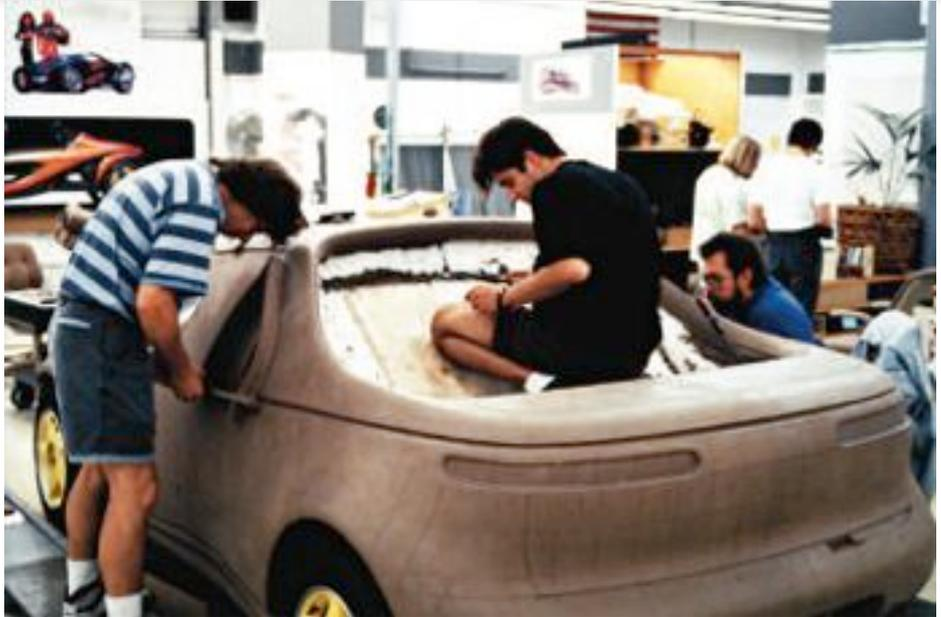
Pontiac design-studio sculptors work on the original clay model, which was used to make the molds for the two show cars. As well as being a concept car, a lot of work went into making this design a feasible production car.
