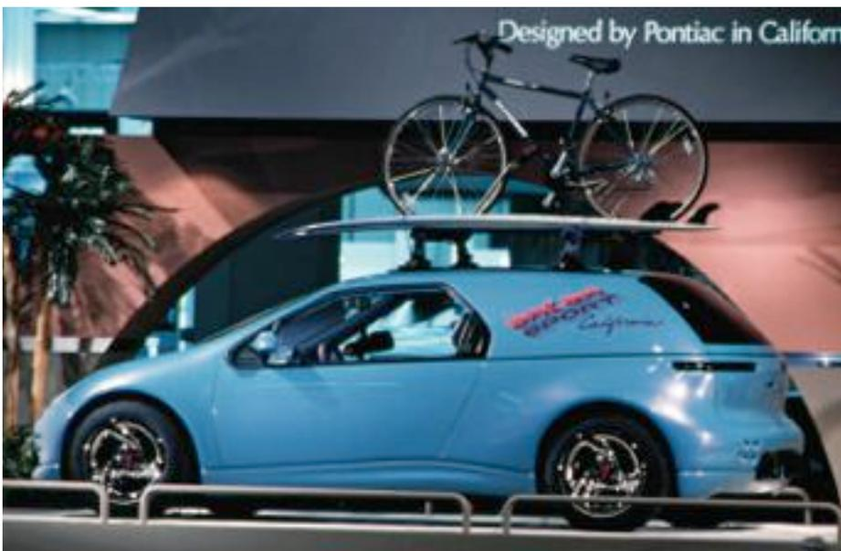
This turquoise panel truck was actually a static model made with fiberglass and wood. It did however have a full interior and was nearly indistinguishable from a fully operational car. It was frequently shown alongside the orange version, which was fully operational.
