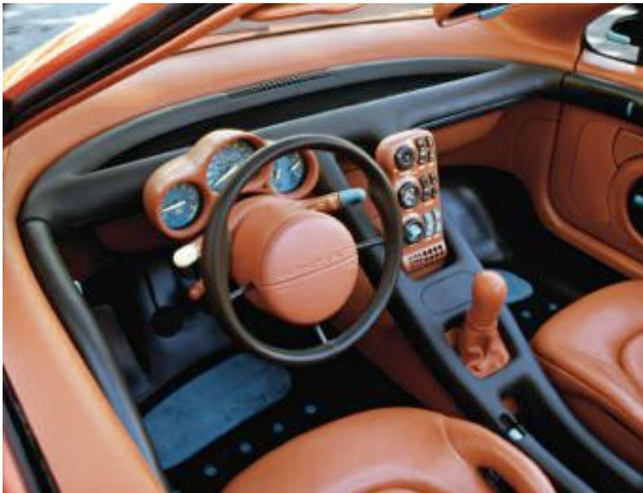
Unique "Crossbow" dash and console design is evident in this shot. Use of earth tones with the bright orange gave a Southwestern feel to the one-off Pontiac. Stereo controls tilt up for easy access. Gauge pod is inspired by motorcycle designs and add to the airy feeling of the interior.
