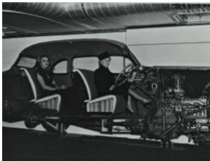
A second 1937 cutaway design was even more severely altered than the first car. This version gave the impression of having been bisected lengthwise with a bandsaw- hopefully those young ladies were not in the car when it happened! Inner details of the engine were revealed and the passenger compartment was fully exposed. Since there were wheels only on the driver's side, the vehicle was supported on the cut line by heavy sections of steel piping that was fastened to a support structure.
